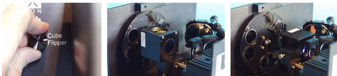
Figure 1 - Cube Flipper Knob, Single Excitation cube position (up), Dual Excitation cube position (down)
