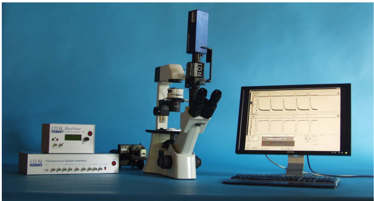
COMPLETE CALCIUM & CONTRACTILITY RECORDING SYSTEM – \mu STEP CONFIGURATION
