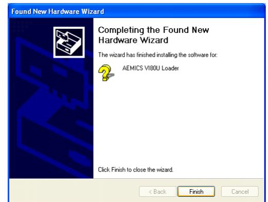
Immediately after you click "Finish", a second "Found New Hardware" popup will be displayed and the "Found New Hardware Wizard" will start again to load the driver for the camera itself. Repeat the process above to load the camera driver.
