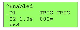
The settings shown above create a situation such that no high voltage output pulses will fire until the rising edge of a TTL signal has been sensed at the "Advance In" input. One pulse will be fired beginning 450 (+/-10) usec after this rising edge, and a second pulse will fire one second later. The pulse train will then remain disabled until another TTL signal is sensed.
