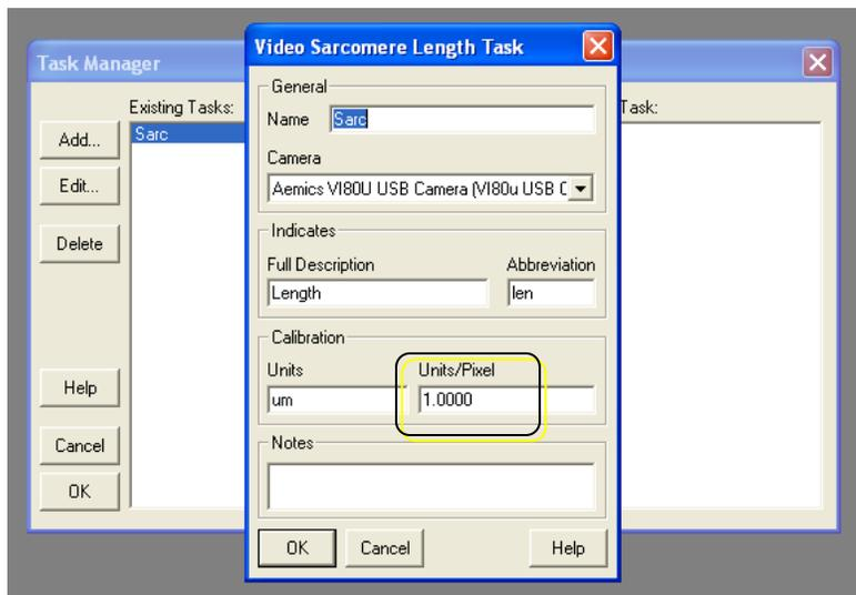
3. Mount and find the micrometer that shipped with your system. Make sure that the micrometer slide is mounted cover glass down. Visualizing the micrometer with the camera's video feed in IonWizard, set the region of interest to encompass a field of micrometer tick marks (you'll want to collect at least 10 tick marks. These tick marks are spaced 10 microns apart.
