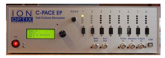
1) Original C-Pace EP. The user is able to select between banks 1 and 2 on the first line of the display, and LEDs and the 9 pin connector are visible in slots 1 and 2. The other slots are blocked by plastic panels.
