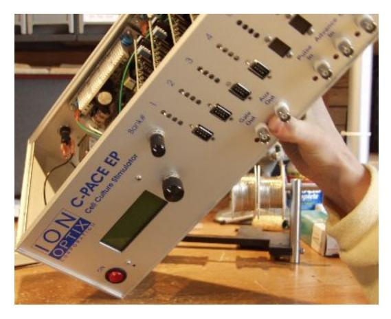
4) Now for the tricky part. It can be difficult to line everything up to fit back into the front panel. The LEDs all have a little give, so make sure they have not twisted or tilted up before you begin. I find it is easiest to hold the main board up and against the panel from underneath with one hand and manipulate the High Voltage Boards and connectors with the other. It also sometimes helps to rest an edge on a table and turn the C-Pace on its side so that gravity is helping.) While
