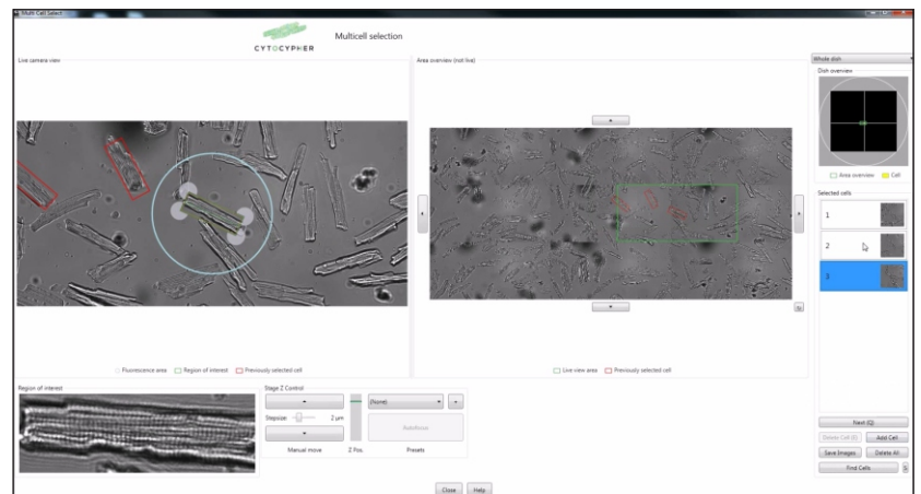
MultiCell myocyte mark-and-find window with digital cell rotation and autofocus
