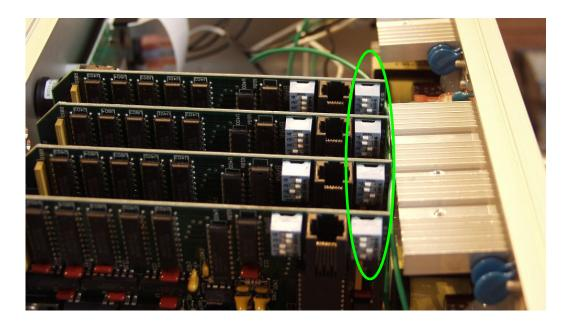
UNPLUG DEVICE! Use a Phillips screwdriver to take the top off the C-Pace or C-Pace EP. You will see the High Voltage Banks mounted vertically. The dip switch closest to the edge of the boards and labeled "WELLS" (circled above in green) sets the dish type the bank is configured to drive. You will see that the settings on the switch correlate to the number labeled on the circuit board.
