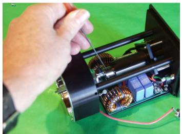
Point the stem of the cathode assembly towards the corner of the housing. This permits its wire to slide in more easily
