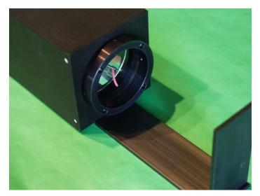
Adjust the 3 silver focusing knobs on the back of the housing to achieve the smallest, centered spot on the Arc Focusing Jig.
