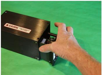
3. Loosen set screw that holds the cathode adapter
