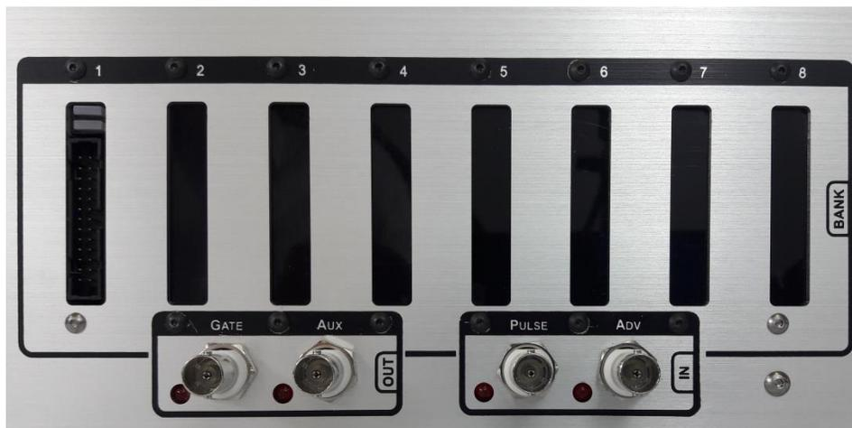
The C-Pace EM supports up to eight independent high voltage banks (HVB). The HVBs can drive either the C-Dish electrode assemblies or the C-Stretch module. The device will automatically recognize whether the C-Dish or the C-Stretch is connected upon initialization.
