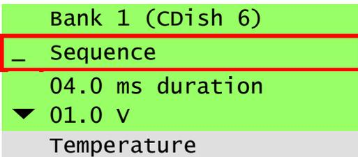
The second line of the Main Menu indicates the Operating Mode of the current bank. There are 3 different modes of operation.
