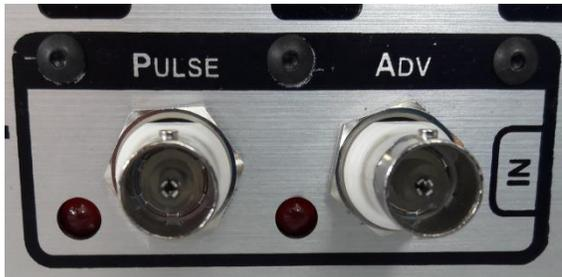
The C-Pace EM has two available digital input BNC connections, **Pulse In** and **Advance ("ADV") In**. These inputs permit other devices to control aspects of the C-Pace EM behavior. These inputs are dedicated to specific purposes as described below.
