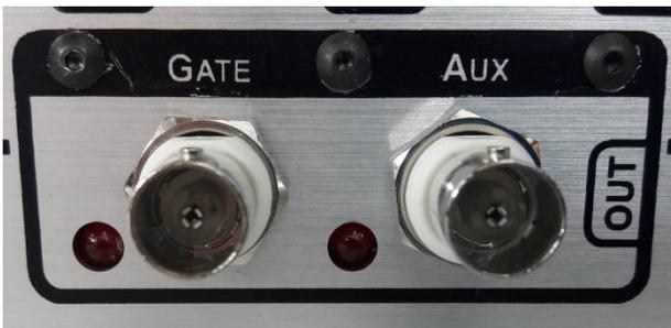
There are two digital output BNC connectors available on the C-Pace EM, **Gate Out** and **Aux Out**. These outputs permit synchronizing other devices to the C-Pace EM via TTL signaling that are timed with the electrical pacing. Both the **Gate Out** and **Aux Out** digital outputs are ultimately synchronized to a single well from a single bank. That well is termed the **Sync Channel**. This well is controlled by the **Sync Channel** setting (see section [3.1.7 below](#)).
