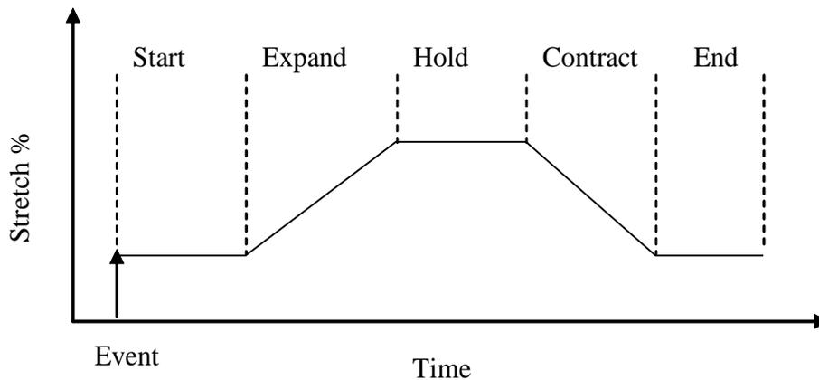
Each cycle begins with the **Start** phase. The length of the chamber at this phase is determined by the **Preload** setting as described below. The cycle then proceeds to the **Expand** phase where the tissue is stretched to a length determined by the **Load** setting. The tissue then rests at the **Load** length during the **Hold** phase. The **Contract** phase is next and returns the tissue to the **Preload** length where it rests for the **End** phase until the next pacer **Event** fires.
