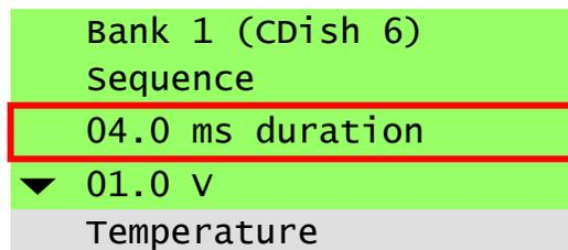
The third line in the Main Menu determines the duration of the biphasic stimulation pulse. The duration of the pulse and can be adjusted between 0.4 and 10 ms for all bank configurations (C-Dish or C-Stretch). The upper range of the duration is dependent on the current pacing frequency, variability settings, and well count and is recomputed when any of those settings change. The bank will reflect the changes as the duration is tuned.
