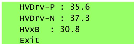
There are several different temperatures shown and an exit option to get you out of this screen. The temperature values, in units of degrees Celsius, are for informational purposes only and cannot be edited. In general, if a particular temperature crosses a threshold that indicates a problem, the system will shut down and indicate an error state with both LEDs showing solid red.
