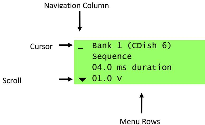
To edit an element on a given row, first turn the **Menu Encoder** knob to move the cursor down the **Navigation Column** to the row in question. Push the knob to select and move the cursor into the row.
