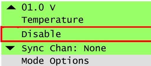
The sixth line in the **Main Menu** enables and disables the electrical pulse trains and (if applicable) the stretch for a bank. When a bank is **Disabled**, reed relays in the high voltage path are opened, ensuring a completely open circuit. These relays are also opened between pulses to prevent leakage of voltage.
