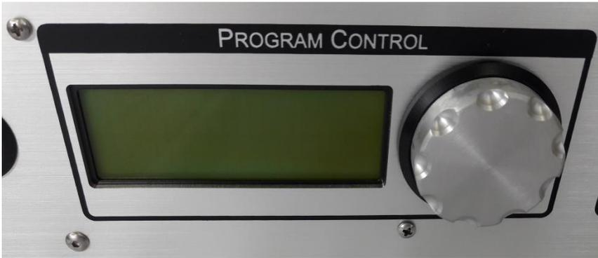
Menu choices and stimuli parameters can be selected via the LCD screen and the **LCD Encoder**, located directly next to the display. To permit one-handed adjustment, the encoder knob can be turned as well as clicked. In general, turning the encoder will perform a scroll function and clicking the dial will perform a select function. Complete documentation on programming the device starts in section [3 Software: LCD Menus](#) below.
