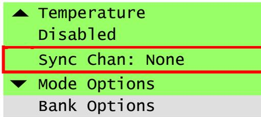
The seventh line in the **Main Menu** is used to set the **Sync Channel** of the entire C-Pace EM device. Both the **Gate Out** and **Aux Out** digital outputs are ultimately synchronized to **Sync Channel** as documented in [2.1.3 Digital Outputs](#) above.
