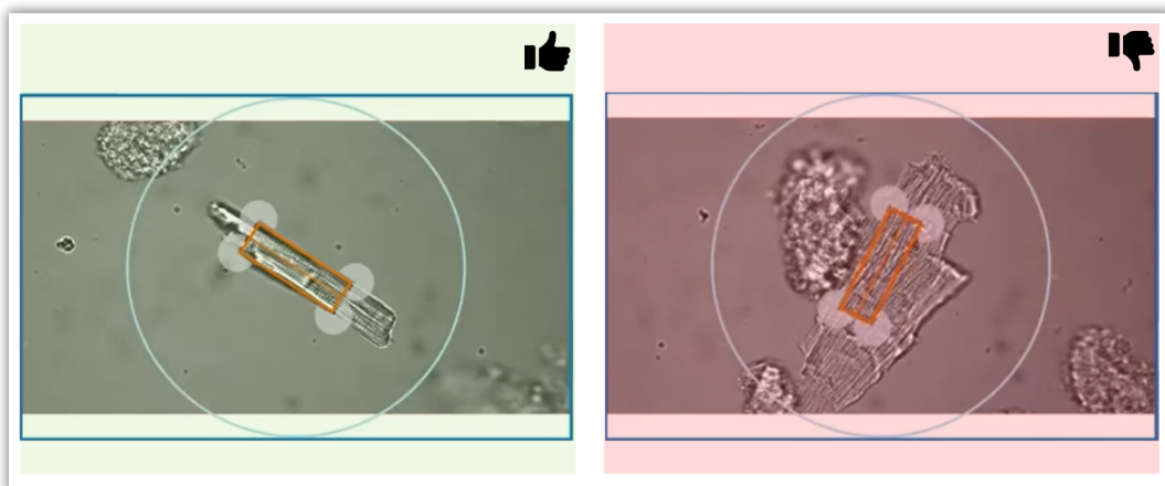
Figure 7: MultiCell HTS and Lite fluorescence illumination. The aperture displaying illumination area is framed by the blue circle shown here. This region should contain only the cell of interest and no debris.
