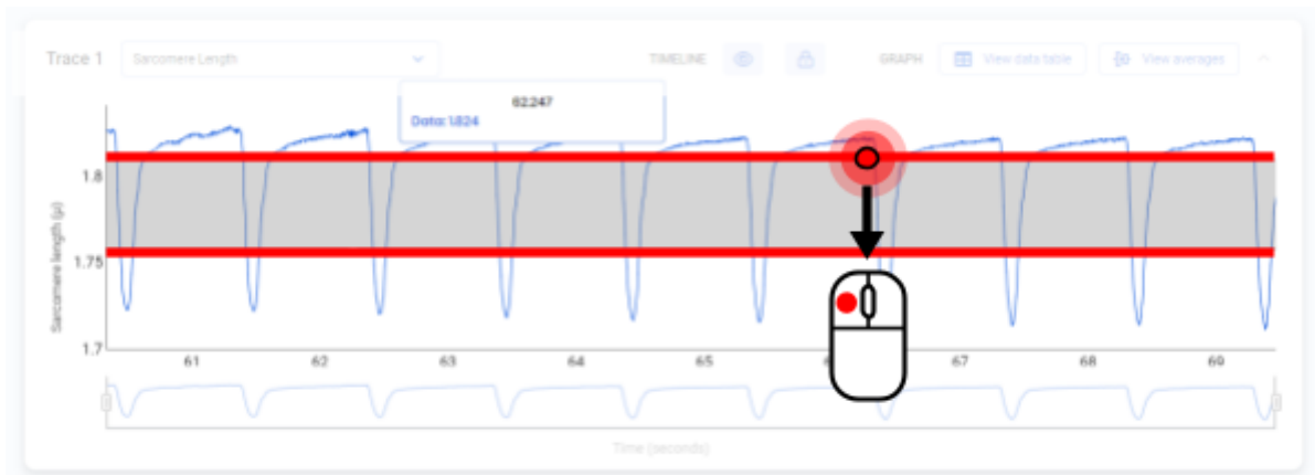
Figure 133. Y-axis zoom by vertically selecting the zoom area.
