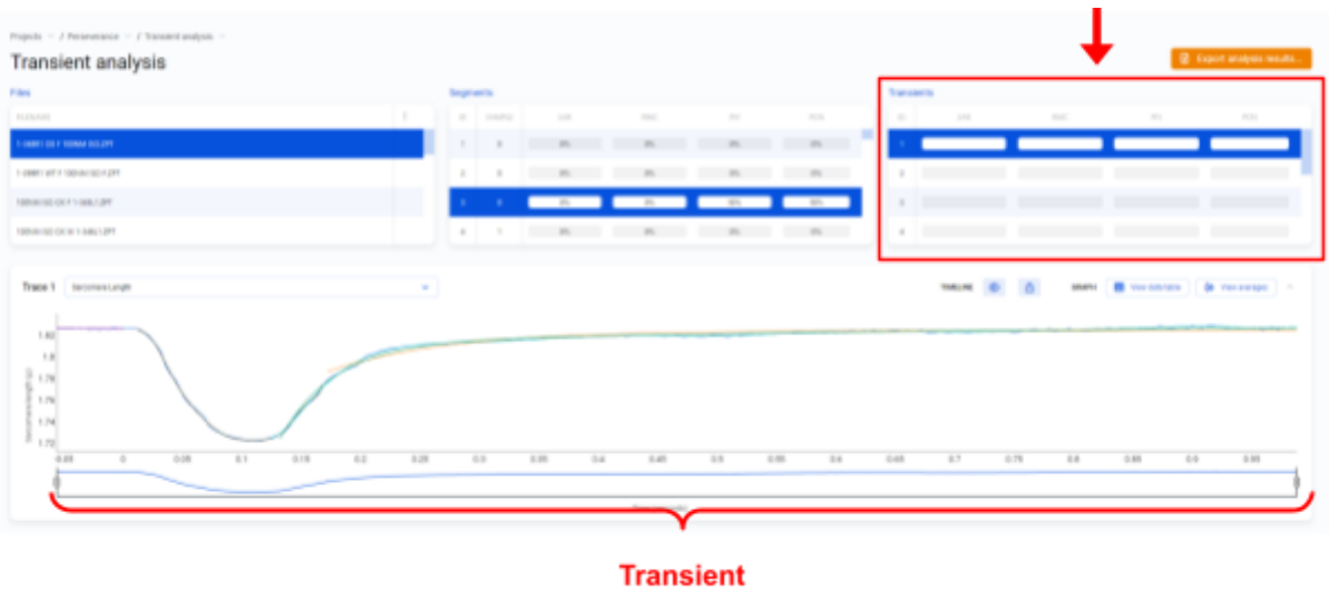
Figure 113. Viewing a segment in Transient Analysis.
